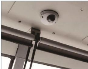
Inward facing cameras are not currently required by U.S. Federal Regulation. However, inward-facing cameras are a key component of a robust safety culture and are an important element for promoting safe train operations. Inward-facing video cameras are another tool for Amtrak and industry regulators to monitor locomotive and engineer performance.
