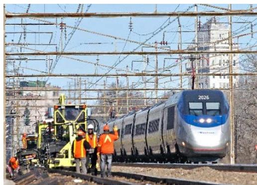
*Amtrak Express trains operate using a catenary system, pictured at top.*
