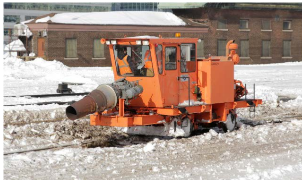
An Amtrak jet-powered snow blower.
