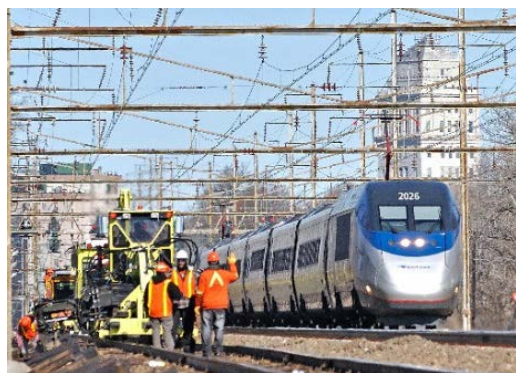
Amtrak Express trains operate using a catenary system, pictured at top.
